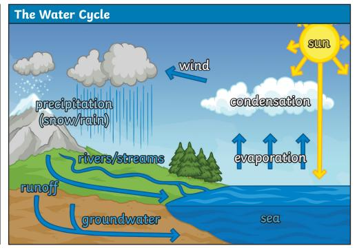
Heat from the sun evaporates water, which rises, condenses in the cool air and then falls back down to earth.
