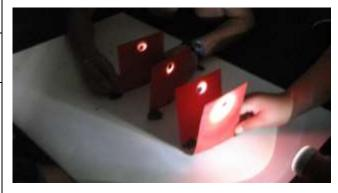
Light reflects off a mirror like a ball hitting a hard surface. The angle it hits the mirror at is the same that it is reflected at.
